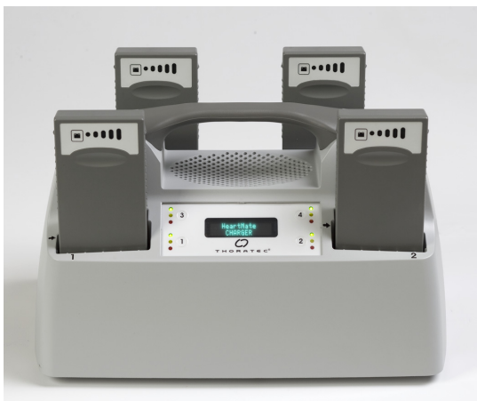
Figure 3.79 Battery Charger with Batteries Inserted in All Pockets
