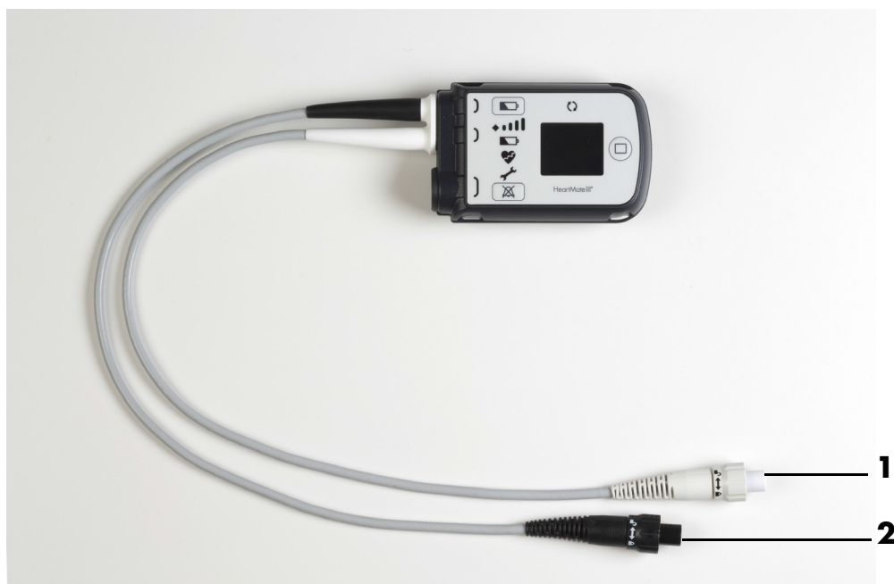
Figure 2.15 Black and White Power Cable Connectors on the System Controller
