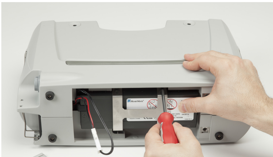
Figure 3.10 Reattaching the Metal Bracket
