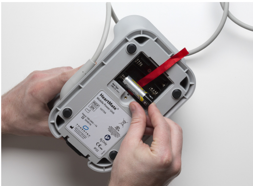
Figure 3.46 Installing the AA Batteries
