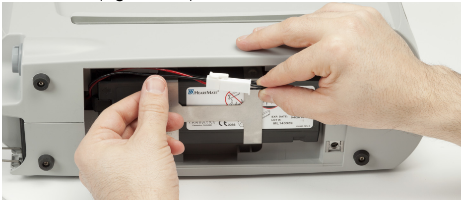
Figure 3.41 Gently Folding the Wires and Connector Along the Top of the Battery
