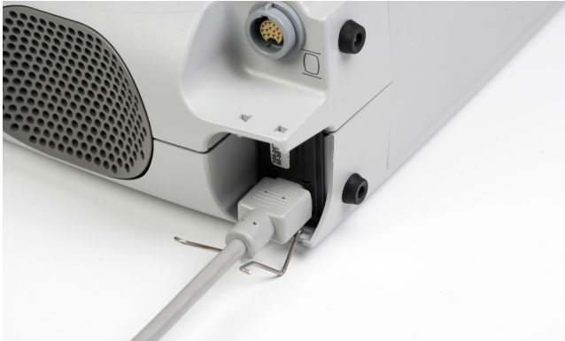
Figure 3.13 Plugging the Power Cord into the Power Module
