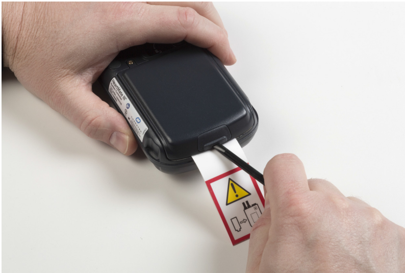
Figure 5.41 Using the Lever to Lift up the Cover
