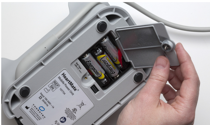
Figure 3.45 Removing the Battery Compartment Cover
