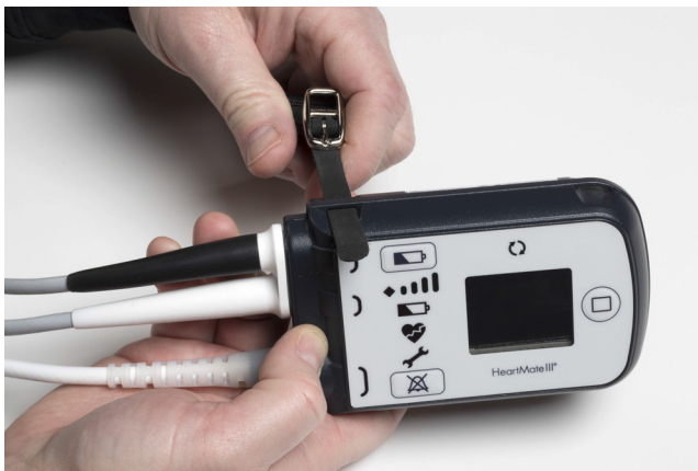
Figure 6.21 Rubber Strap Through the Attachment Point
