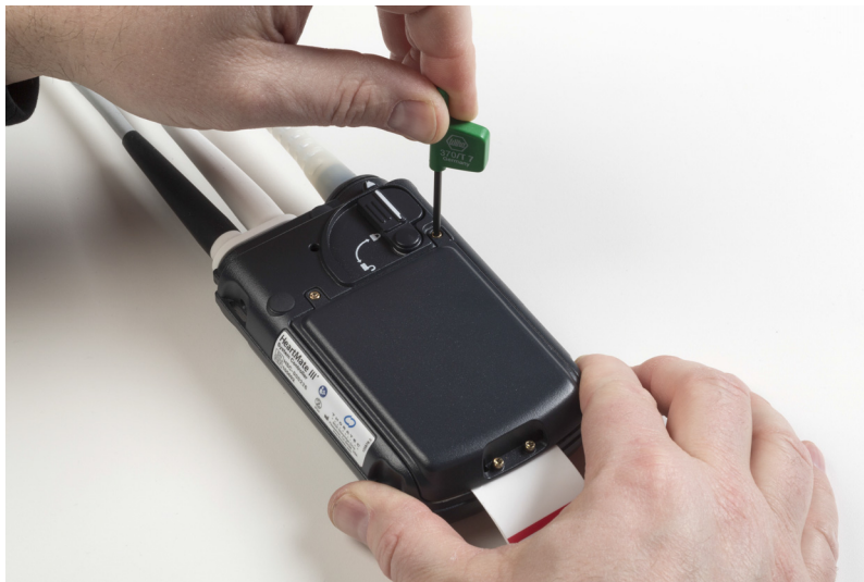
Figure 5.42 Loosening the Screws
