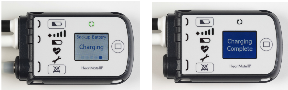
Figure 2.35 System Controller Charging or Charging Complete
