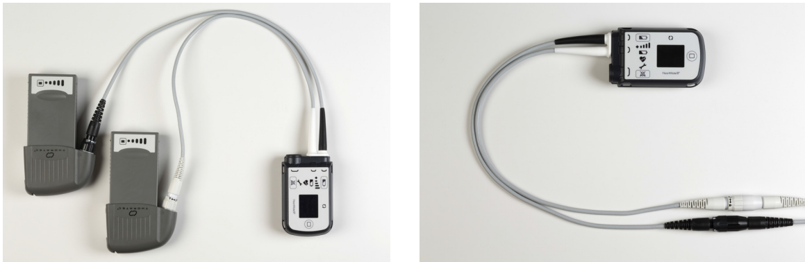
Figure 2.21 System Controller in Charge Mode While on Battery Power (left) and the Power Module (right)
