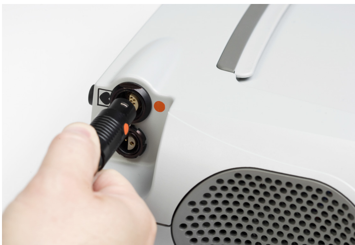
Figure 3.17 Aligning the Red Dots
