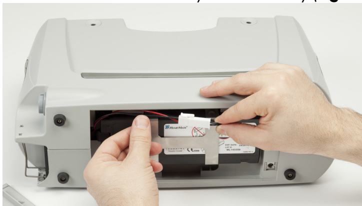
Figure 3.33 Gently Pulling the Wires and Connectors Away From the Battery
