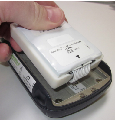
Figure 5.44 Placing the Battery Inside the Compartment
