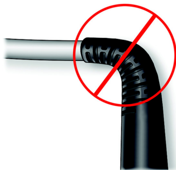
Figure 6.1 Do Not Bend System Controller Power Cables
