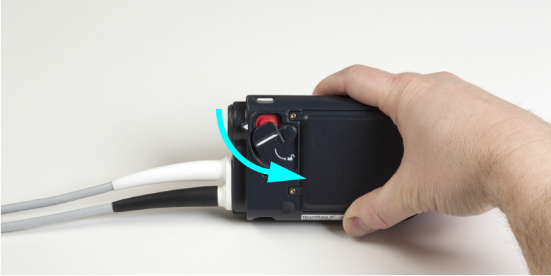
Figure 2.10 Unlocking the Safety Lock
