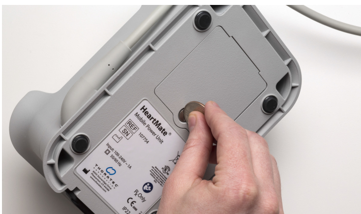
Figure 3.44 Loosening the Screw
