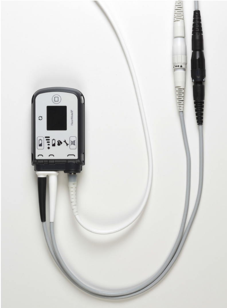
Figure 3.26 System Controller Power Cables Connected to Power Module Patient Cables
