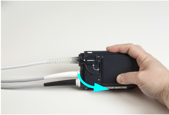
Figure 2.42 Unlocking the Safety Lock
