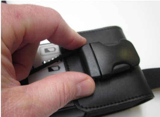
Figure 6.29 Clip the Strap Into Place
