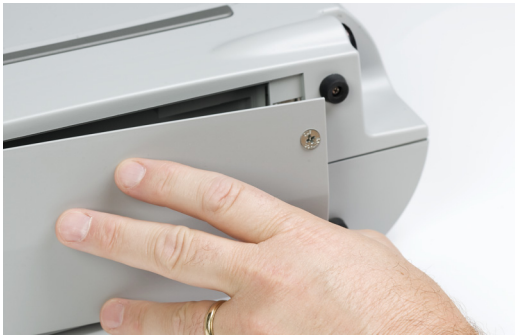
Figure 3.6 Removing the Battery Compartment Cover
