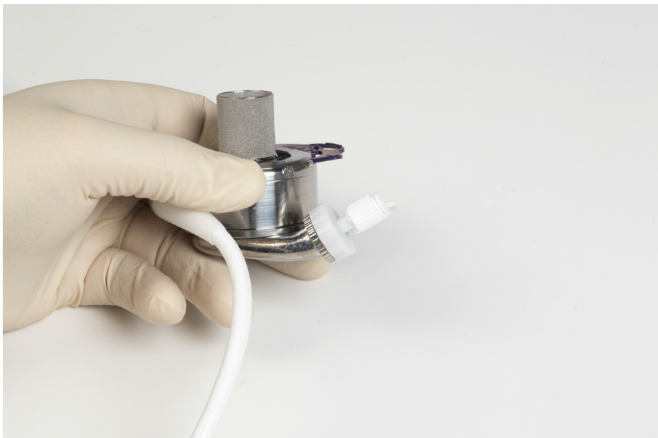
Figure 5.23 Attaching the Luer-Lok Connector to the Pump Outlet
