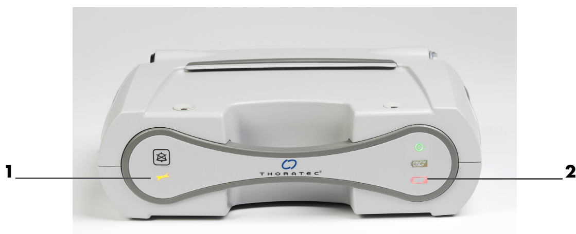
Figure 3.30 Yellow Wrench and Red Battery Hazard Symbol (Power Module Backup Battery is Not Working)
