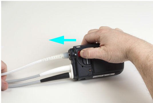
Figure 2.54 Removing the Driveline
