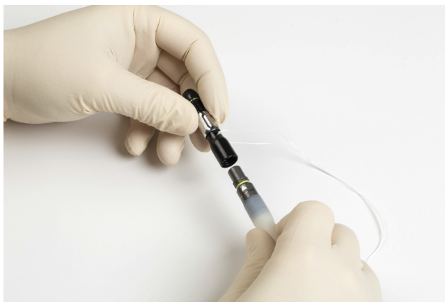
Figure 5.22 Attaching the Tunneling Adapter to the Pump Cable
