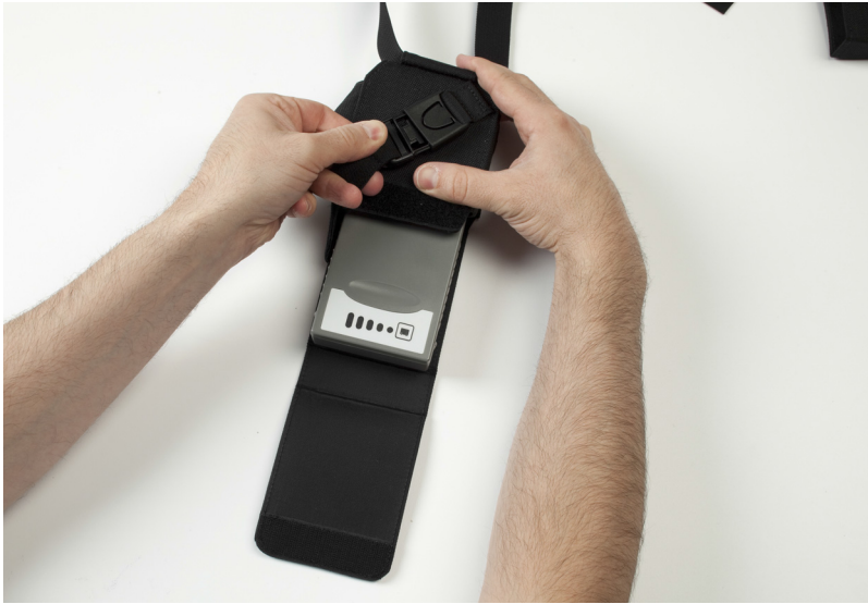
Figure 6.51 Buckle the Clip on the Holster
