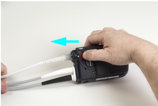
Figure 2.43 Removing the Driveline
