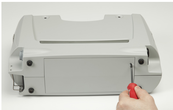
Figure 3.31 Loosening the Screws
