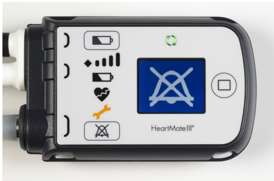
Figure 7.3 Sample Alarm Silence Indicator
