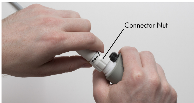
Figure 7.8 Turn Nut on the Connector
