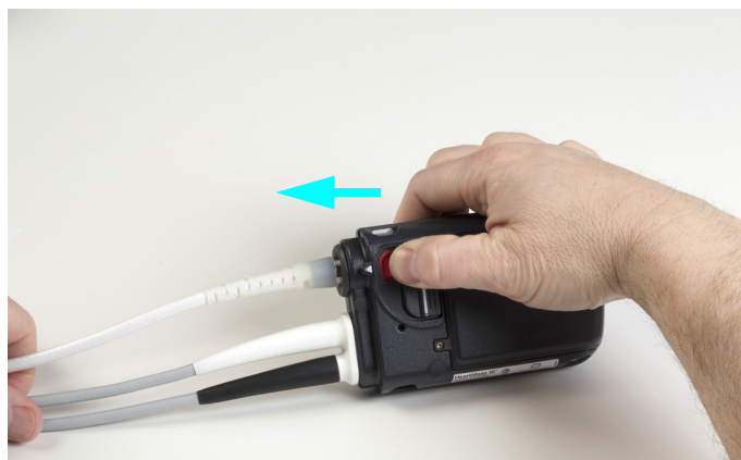
Figure 2.14 Removing the Driveline
