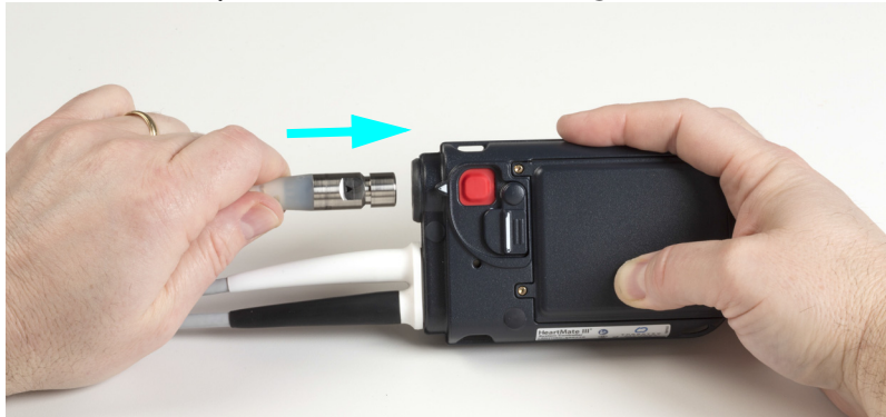
Figure 2.11 Aligning the Arrows
