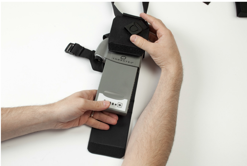
Figure 6.50 Inserting Battery and Clip into Holster
