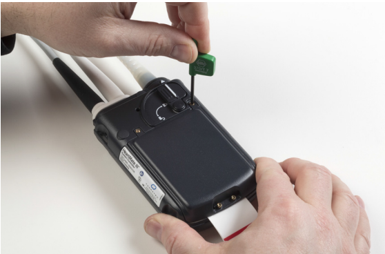
Figure 2.26 Using the Screwdriver to Loosen the Screws
