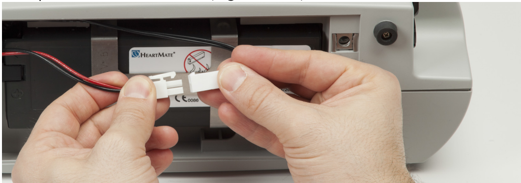
Figure 3.40 Lining Up the Connector Halves
