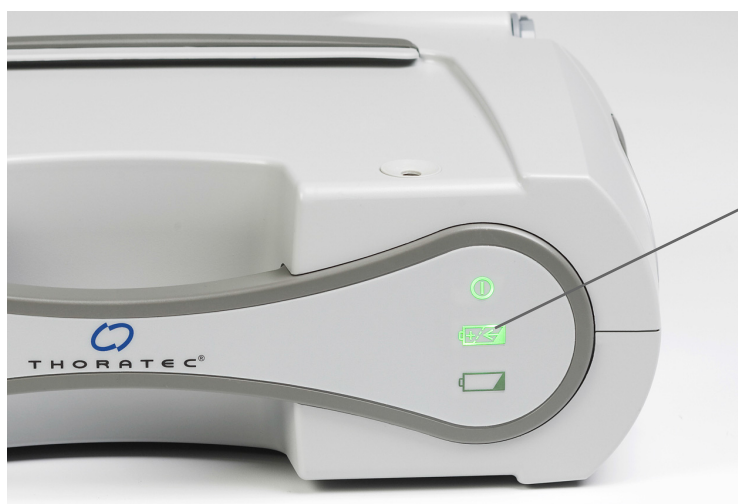
Figure 3.27 Green Charge Symbol (Power Module Backup Battery is Charged)
