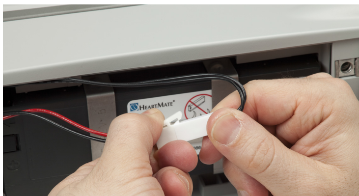
Figure 3.34 Gently Squeezing the Latch
