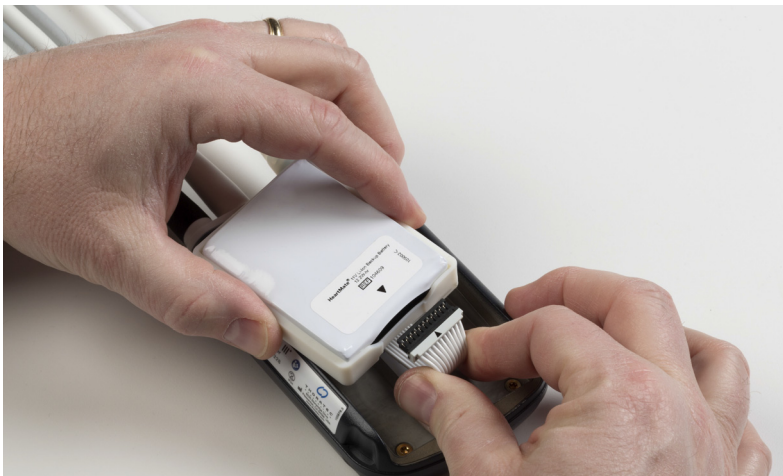
Figure 2.32 Installing the Backup Battery
