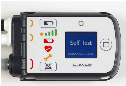
Figure 2.17 User Interface During System Controller Self Test
