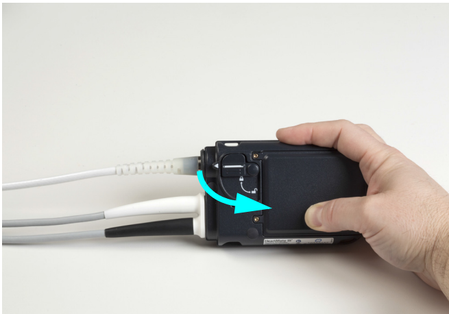
Figure 2.13 Unlocking the Safety Lock
