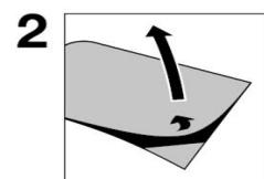
Peel off the backing foil and remove the capsule.
