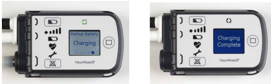
Figure 2.26 System Controller Charging, Charging Complete
