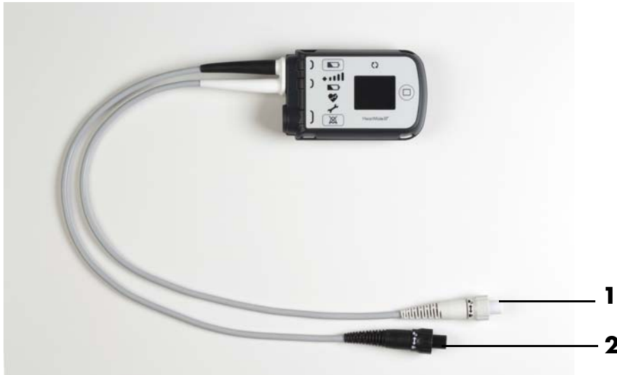
Figure 3.23 System Controller Power Cables With Black and White Connectors
