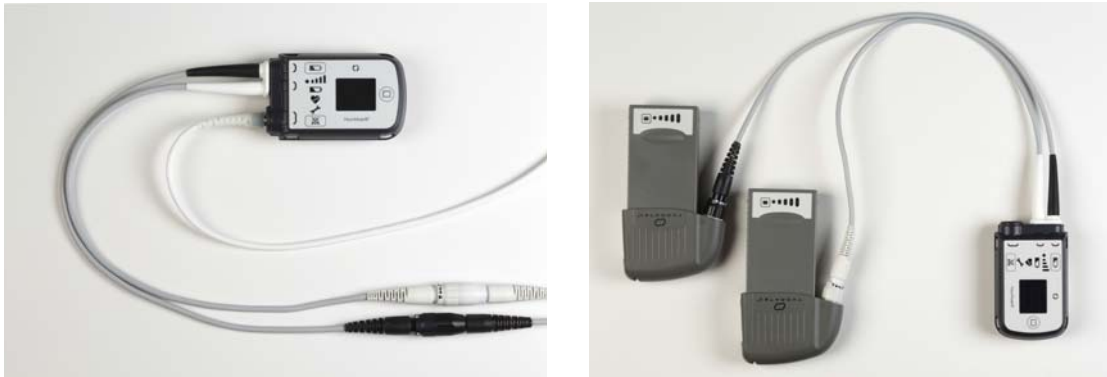
Figure 2.25 System Controller on Mobile Power Unit Power (left) and Battery Power (right)
