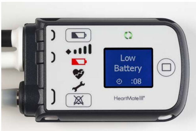
Figure 2.20 Low Battery Power Alarm (Less Than 5 Minutes of Power Remain)
