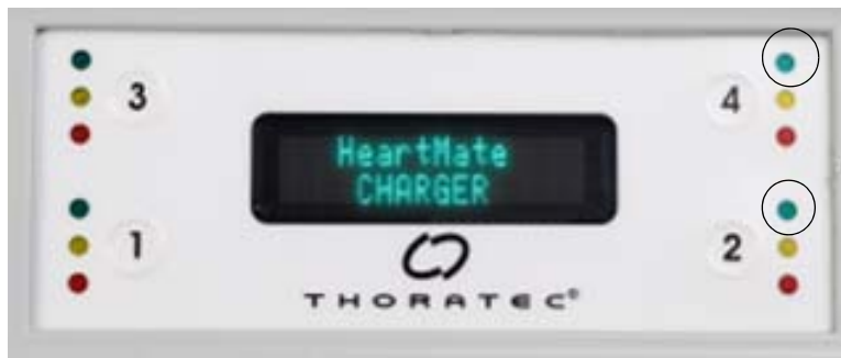
Figure 3.32 Green Light Indicating a Charged Battery
