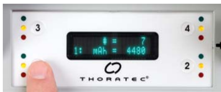
Figure 3.39 Press the Button a Second Time to Display Battery Charge Cycle Information
