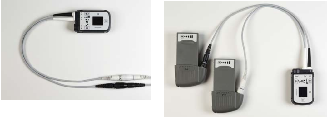
Figure 2.23 System Controller in Charge Mode: Mobile Power Unit Power (left), Fully-Charged Batteries (right)
