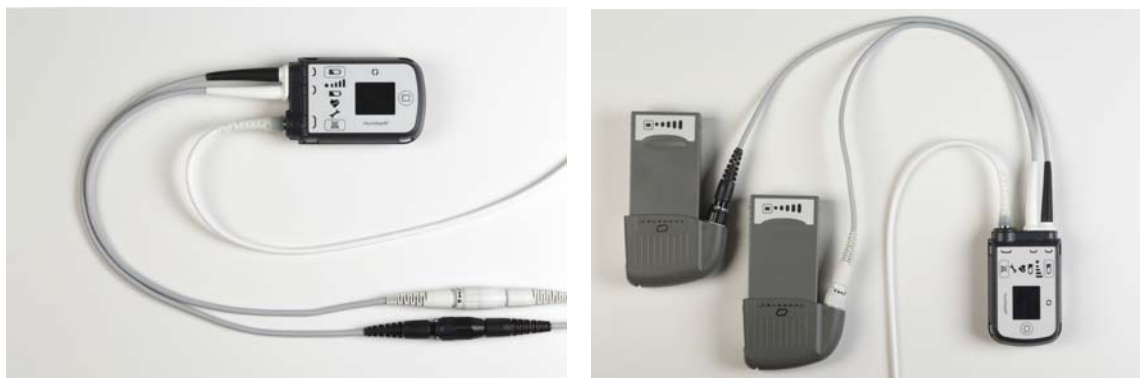
Figure 2.21 System Controller in Run Mode While Connected to the Mobile Power Unit (left) and to Batteries (right)
